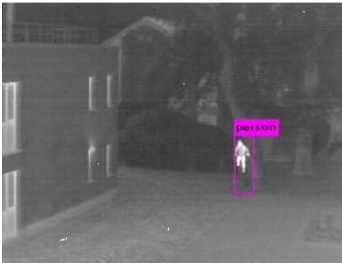
Example of the infrared camera taking images in the dark. The person is clearly visible despite the difficult external conditions.
